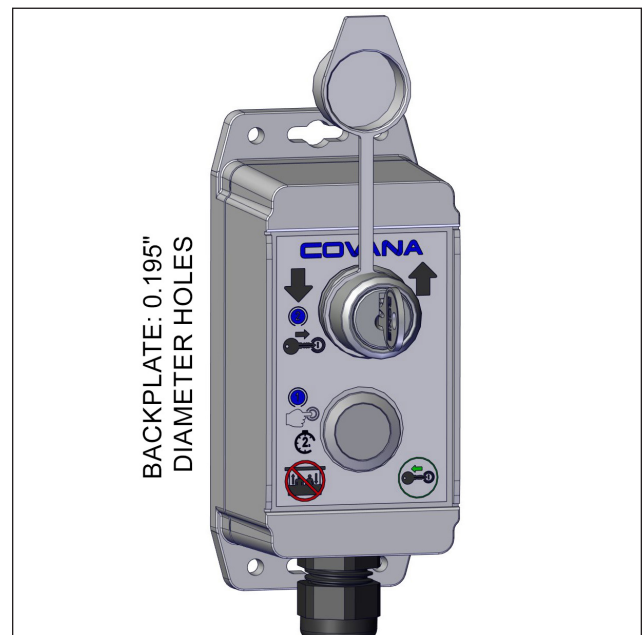
FIGURE 54: OR FASTEN BACKPLATE OF KEY SWITCH WITH TWO SCREWS (NOT INCLUDED)
