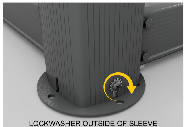
FIGURE 34: TIGHTEN SCREW ON EACH SLEEVE
