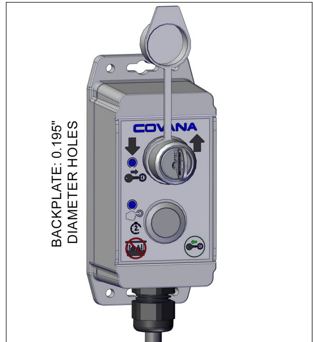
FIGURE 52: OR FASTEN BACKPLATE OF KEY SWITCH WITH TWO SCREWS (NOT INCLUDED)
