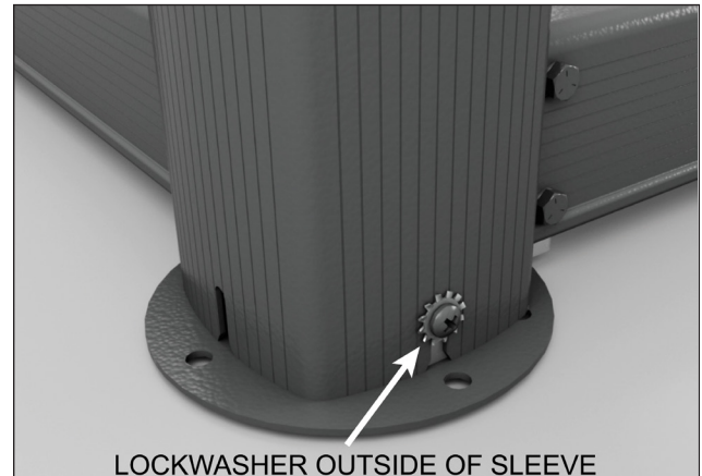
FIGURE 93: LOWER THE SLEEVE AND TIGHTEN THE SCREW
