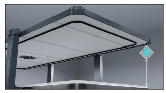
FIGURE 108: APPLY 15 PSI PRESSURE WITH J-ROLLER
