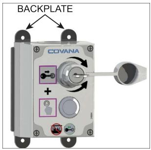
FIGURE 49: FASTEN THE BACKPLATE WITH FOUR SCREWS
